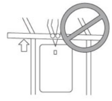
Do not pull the wiring cables or junction box
